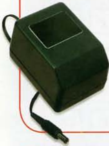
AC adaptor (Optional) Input 110 or 220 VAC Output 13.80 VDC at 800 mA
